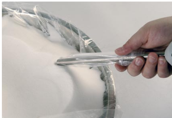
Figure2: Sampling by direct contact
